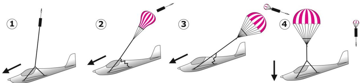
This system is equipped with a parachute canopy, which in most cases is pulled up using a solid fuel rocket engine. The parachute canopy is connected to the aircraft by a suspension system (steel ropes/straps).
