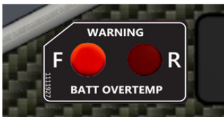
Example: front (F) battery overtemp warning light active
