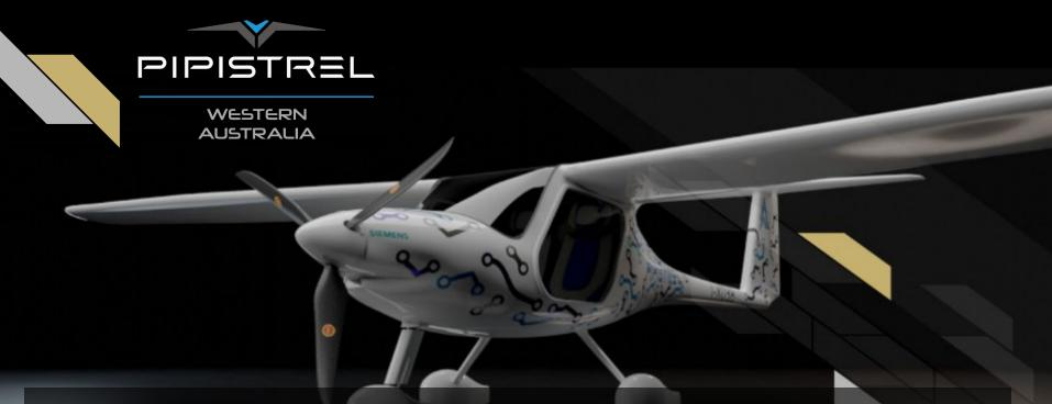
The Pipistrel Alpha Electro is a 2-seat electric trainer with performance which is tailored to the needs of flight schools. It has short take-off distance, powerful 1000+ fpm climb capability and an endurance of one hour plus a 30-minute reserve. The Alpha Electro is optimized for traffic-pattern operations, where up to 13% of energy is recuperated on every approach, increasing operations range and at the same time enabling short-field landings.
