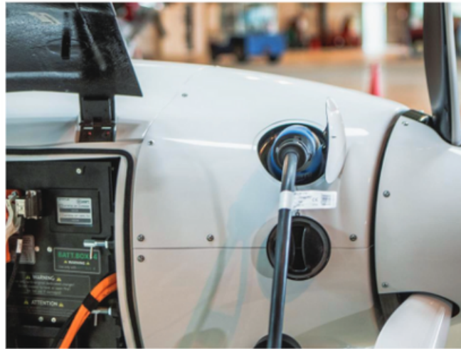
Charging plug-receptacle interface (Example Alpha Electro)
